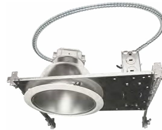
8120H 4" LED Frame-In Size: 12-1/6" x 7-5/8" x 4-7/8" Opening: 4-13/16"
