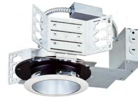
8124H 6" LED Architectural Housing Size: 12-3/8" x 7-7/8" x 6-3/4" Opening: 6-3/8"
